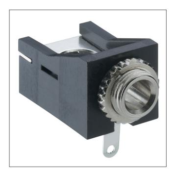
Jack chassis socket acc. to JIS C 6560 JC35J2B, 3.5 mm, 2 poles/mono, angular version, with break contact and solder eyes, for printed circuit boards, for back side mounting
